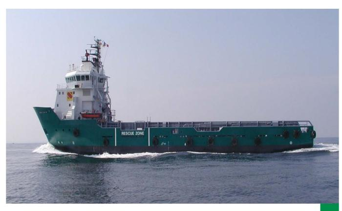
The is an UT 755L design, DPI, FIFI 1, platform support vessel.
